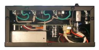
The reactor component inside a Zero Surge unit is made from 10 gauge copper wire (a heavier gauge than 15 or 20 amp house wiring). There is less copper wire in a Zero Surge unit than between the local distribution transformer and your equipment! Any slight variation in voltage will be less than
