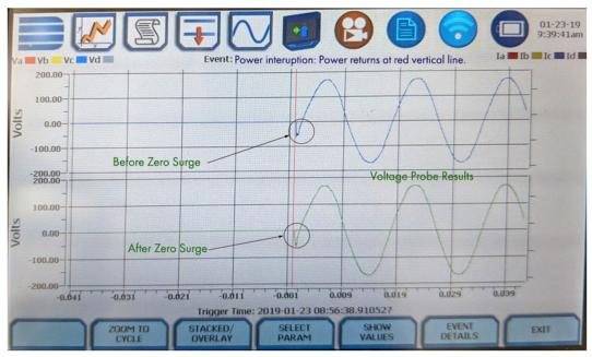
Figure 1: Voltage Probe Results
