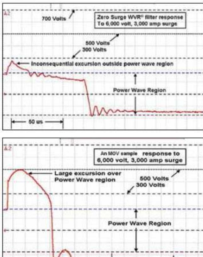
*Two oscillographs of surge suppressors reacting to an incoming surge of 6000 volts and 3000 amps. Note the total time outside the power wave is high for the MOV.*
