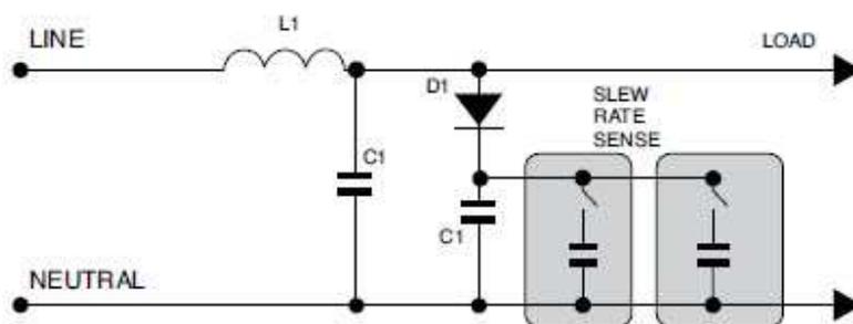
*Simplified schematic of a series mode filter. There are no sacrificial components, so the filter does not wear down with use, and it repeatedly eliminates surges.*
