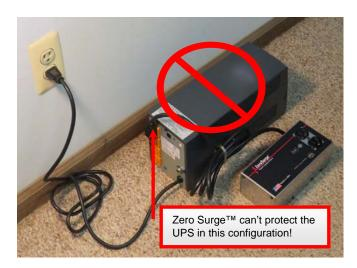
When using Zero Surge products with a UPS, the Zero Surge unit must be ahead of the UPS to protect the UPS and its connected equipment. Simply plug the Zero Surge unit into the wall outlet, plug the UPS into the Zero Surge unit, and plug the sensitive electronics into the UPS. This will also insure that the MOVs inside the UPS remain dormant, preventing ground line contamination.
