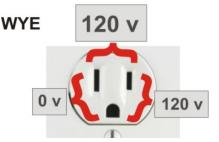
A marine electrical professional using a voltmeter on a WYE wired circuit will read voltage across the terminals as shown in the image on the left. For a WYE configuration 120 VAC is established between the hot terminal and the neutral terminal *and* the hot terminal and the ground terminal of the receptacle.
