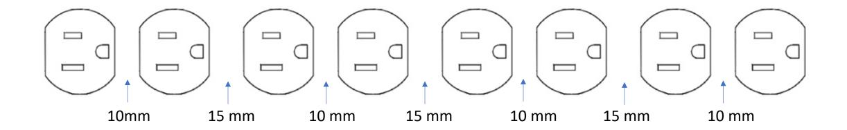
Spacing for the rack mounted products are based on sets of duplex receptacles. The 10 mm is the space between a duplex receptacle (used in all of our products) and the 15 mm spacing is between each set of duplex receptacles. For 10R products, the spacing between the two receptacles is 10 mm.
